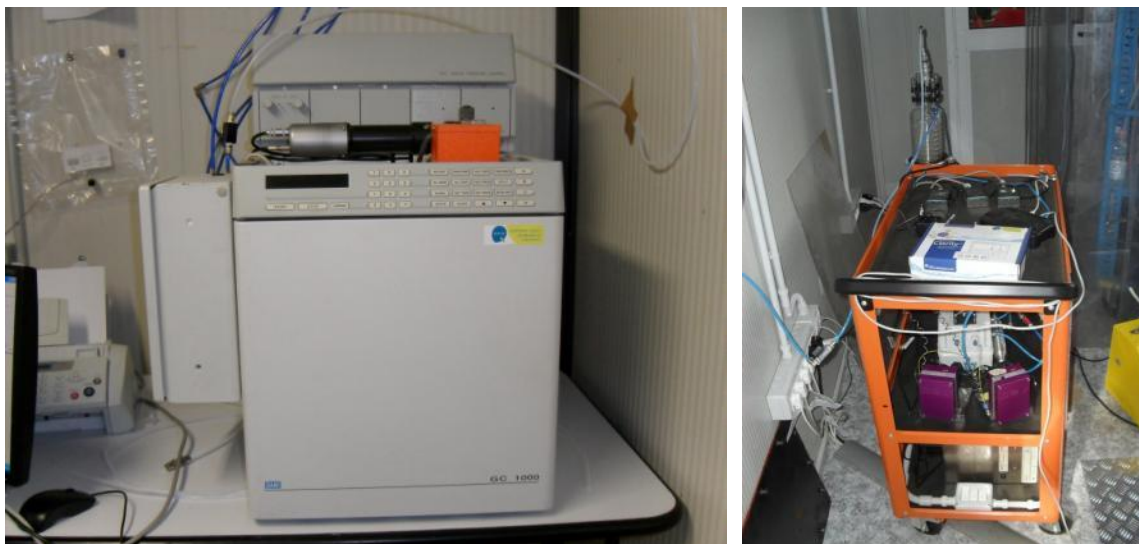
GC system for pollutant measure (GC DANI) and for online gas analysis (C2V)
