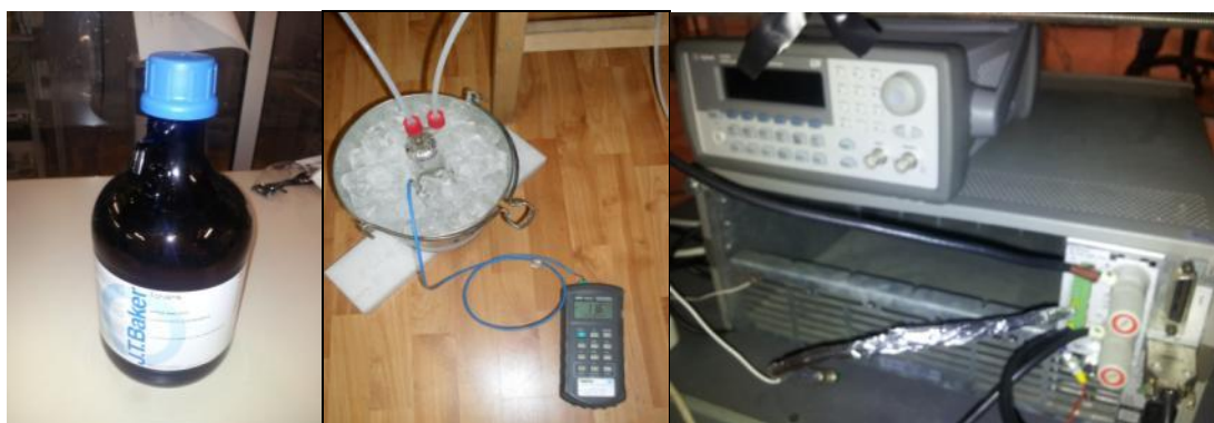
System developed to perform toluene pollution and EIS set-up
