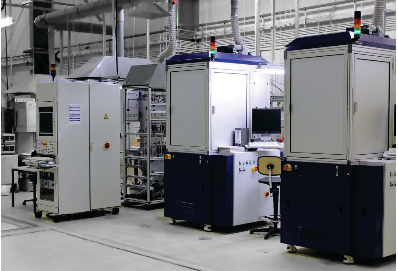
Figure 3: New test benches for single cells of 16 cm 2 at Forschungszentrum Jülich with cell current up to 40 A.
