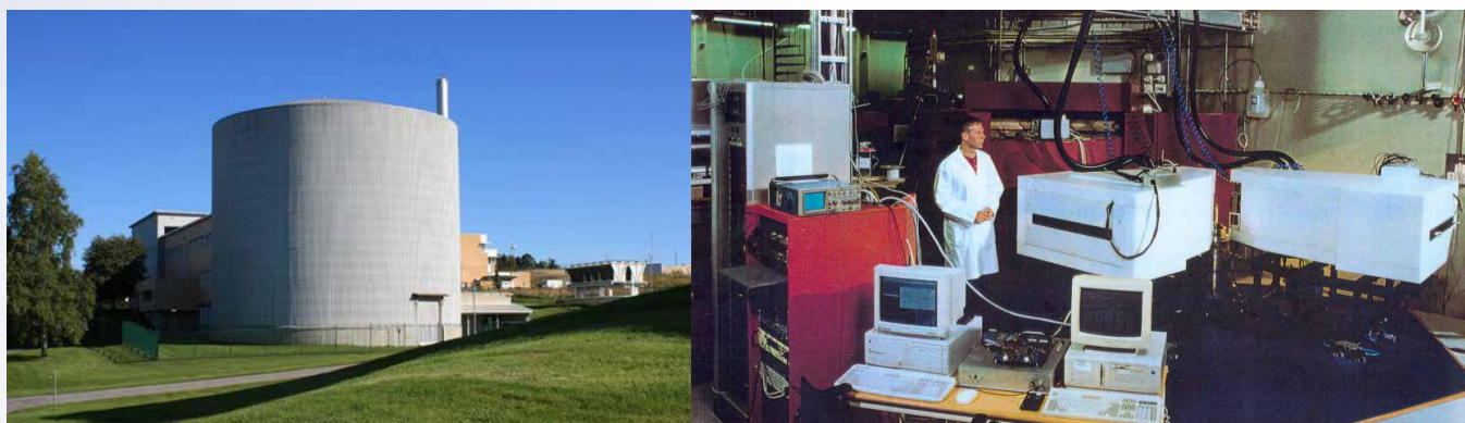
Figure 2: a) The JEEP II reactor operated by IFE (Kjeller, Norway) is a neutron source for material science. b) The neutron diffractometer PUS at JEEP II is suitable to determine the structure of hydrogen-containing materials.
