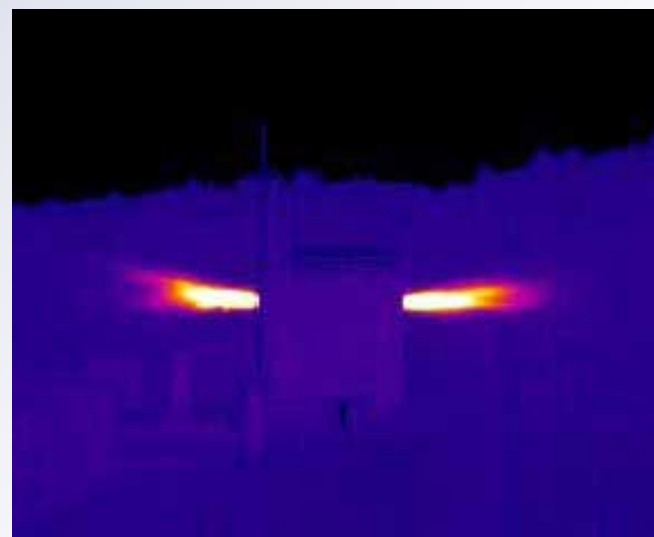
Figure 3: IR image of vented deflagration through passive vents
