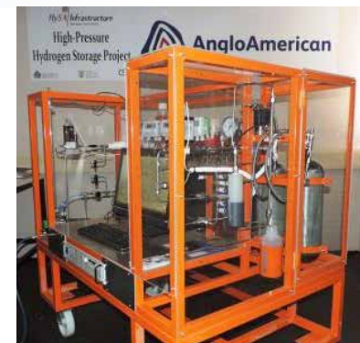
Figure 3: Fully functional EHC system prototype developed by HySA Infrastructure.
