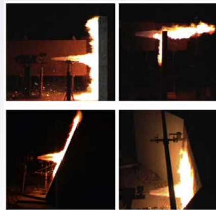
Figure 6: Impinging jet fire [2]
