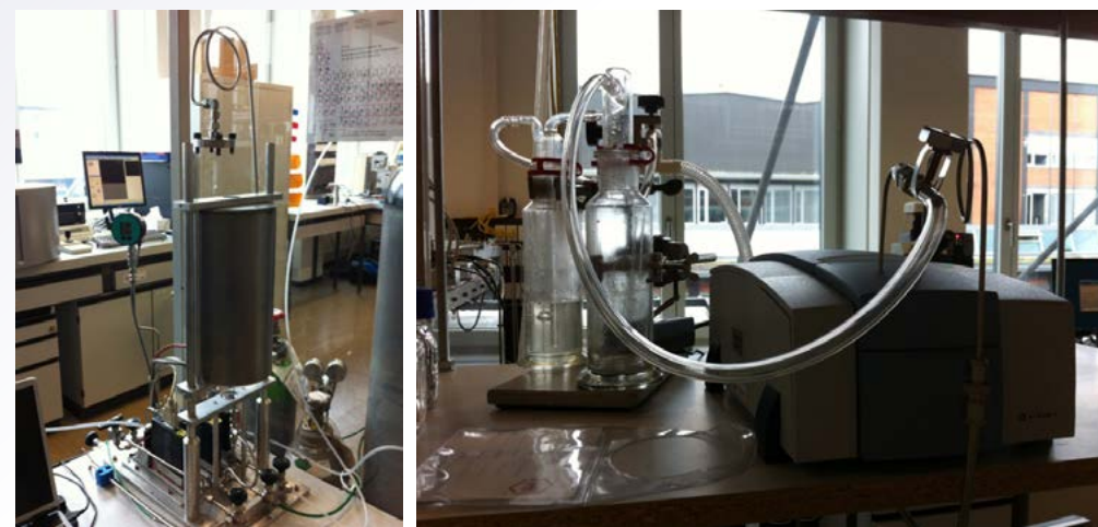
Fig. 2: Reactor for catalytic reactions (left) and IR spectrometer, monitoring the gaseous species.
