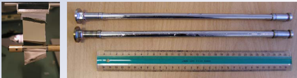
Figure 2: Hydrogen separation membranes prepared from thin Pd-alloy foils.
