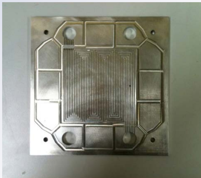
Figure 2: 316L stainless steel flowfield plate with hole for in situ probe.
