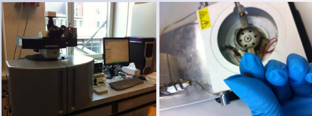
Fig. 1: Raman setup (left) and Raman cell for high pressure experiments (right).
