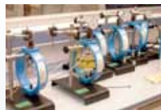
Hydrogen Assisted Stress cracking testing configuration based on dynamometric rings
