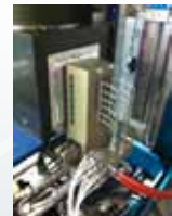
The ECL setup for simultaneous operation and imaging of 6 fuel cells, in the ICON beam line
